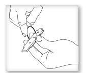
v. Feed the wires through the holes in the ceiling tile.
